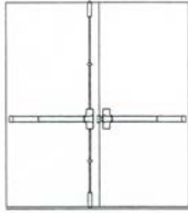
Rim Device and SVR or CVR Device combination – same direction. Overlapping astragal is not required. Coordinator with double door strike is required.
